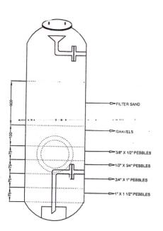
Typical Layout of Sand and Carbon Filter
