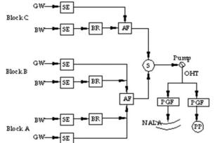
GW-Grey Water, BW-Black Water, SE-Settler, BR-Baffle reactor, AF-Anaerobic Filter, PGF-Planted Gravel Filter, PP-Polishing Pond
