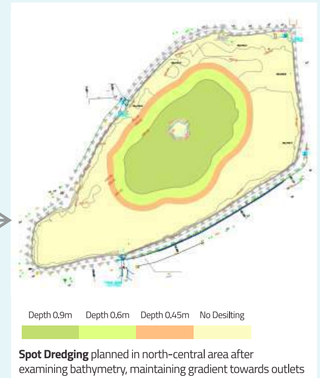
Proposed Plan for Desilting in Selvachintamani Lake , Coimbatore
